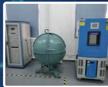
光谱测试仪+高低温测试仪 Spectroscopy tester+ High and low temperature tester
